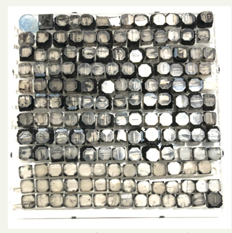
Diamonds mounted in the laser system ready to be analysed to check their origin.
